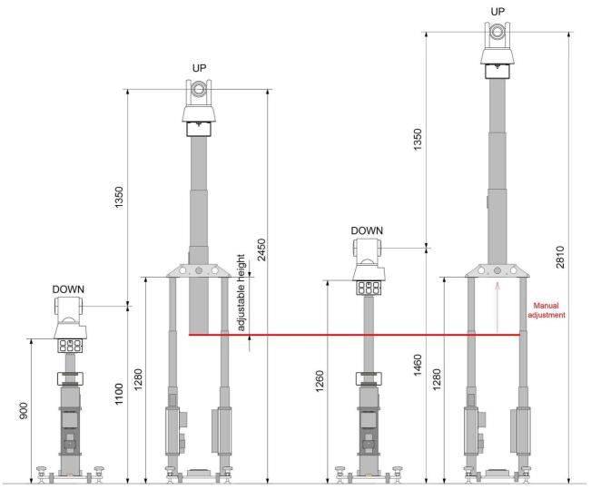
The difference between the two configurations is the manual adjustment of the central column.
